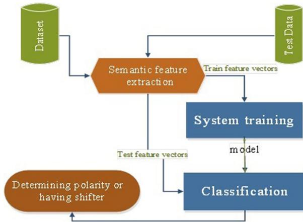
**Fig. 2** Flowchart of a semantic-based machine learning system
